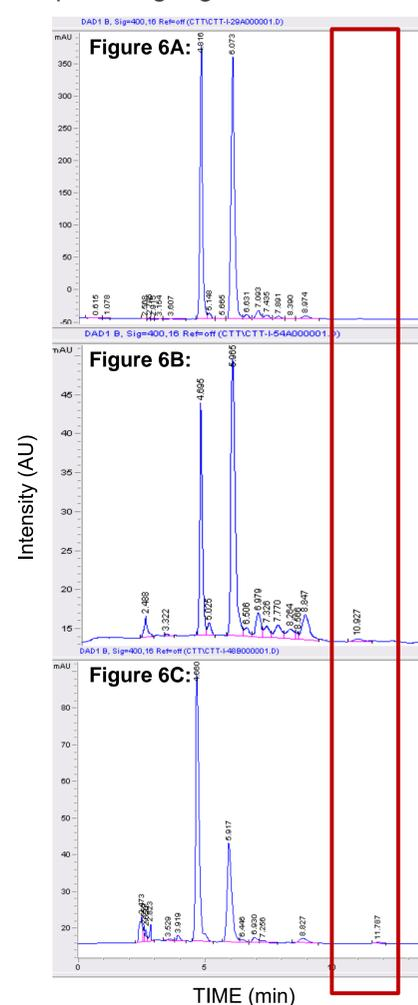
Figure 6: HPLC chromatograms for a mixed empty fullerene standard (Fig. 6A),  $Sc_2O_3$  composite rod soot (Fig. 6B), and  $Gd_2O_3$  composite rod soot (Fig. 6C).
