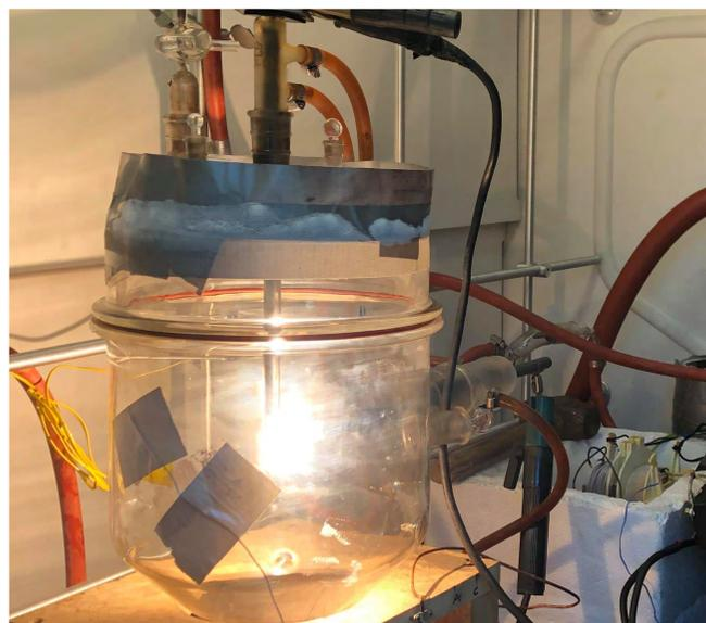
Figure 4: Arc vapor deposition reactor. The packed graphite rod (anode) is parallel to the ground, while a simple graphite cathode is perpendicular to the ground. A plasma arc is observable between the two electrodes. This method produces both empty and filled fullerenes.
