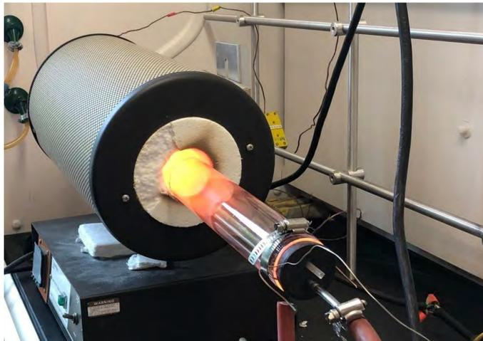
Figure 3: Tube furnace setup for curing packed rods. The gas inlet fills the quartz tube with helium gas in order to maintain an inert atmosphere and prevent oxidation of the graphite.
