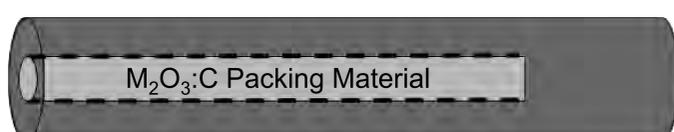
Figure 2: Diagram of a packed graphite rod. Figure not to scale.
