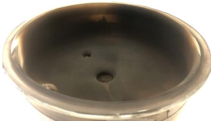
Figure 5: Soot deposit from the combustion of a  $Sc_2O_3$  packed rod.
